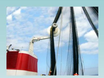
Net Crane type NK-6000T is designed to make the net and cork line stacking easier on tuna vessels, where the net is hauled from the sea by a power block in a boom.
