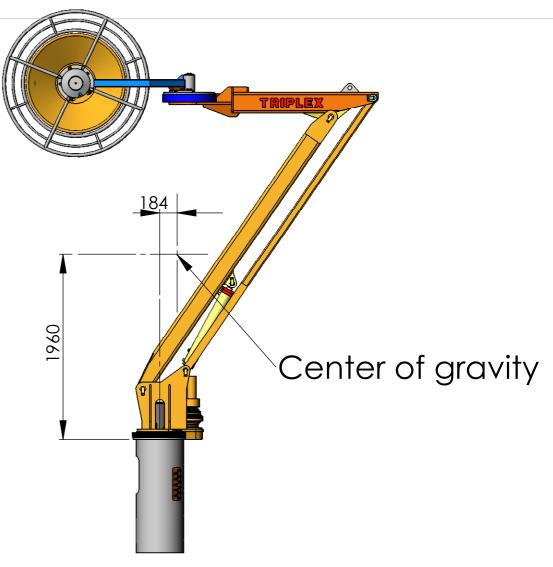
Max working radius 5,52 m Turning angle 360 deg Working head slewing torque 1500 Nm Working head turning angle 260 deg Working pressure 200 bar Recommended oil supply 45 I/min Required powers for oil pump 18 kW Max. Hauling power roller 1500 N Slewing torque crane 10 kNm Weight without foundation approx. 1155 kg Weight foundation approx. 210 kg/m
